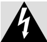
The arrow-end lightning symbol inside the equilateral triangle informs that in the context of the product, there is enough amount of 'uninsulated' dangerous voltage to cause an electric shock.
